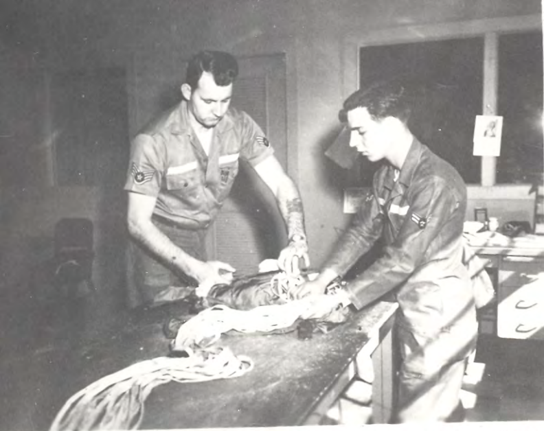
An average of 40 to 50 F-100 drag chutes are packed daily at the MBAFB parachute shop. A2C Albert W. Hedley (r) uses a hook for packing. SSgt. Walter Cole expertly places shroud lines into the canvas pack.
