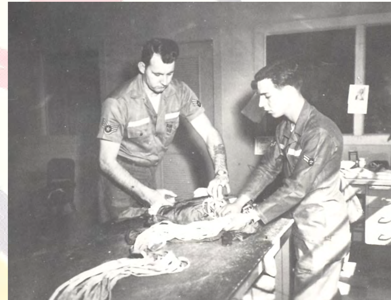
On average 40, to 50 F-100 drag chutes were packed at the Parachute Shop. A2C Albert Nedley (r) uses a hook for packing.
