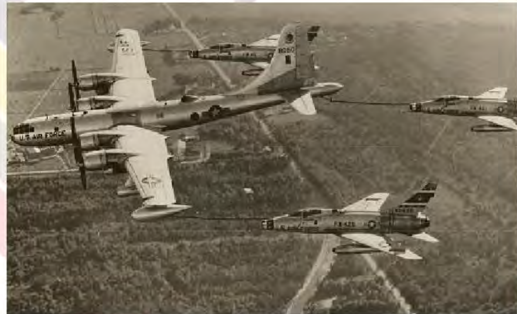
B-29s, and later B-50s, were retrofitted so that they could be used as aerial tankers. Refueling hoses fitted with a drogue, a basket-like device about two feet in diameter, could be unreeled from the tanker. The pilot in the fighter then connected a probe to the drogue. Above, a KB-50J refuels three F-100 Super Sabres.
